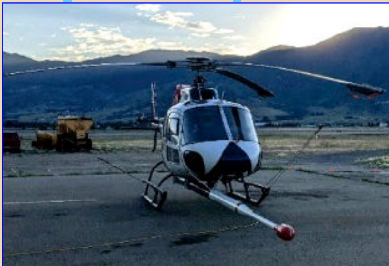
Fig. 4. The survey helicopter (parked at Bert Mooney Airport east of Butte, Montana) used to create the magnetic survey map of Fig. 3. The measuring equipment used is a 'magnetometer' rigged on a fiberglass boom placed at the front of the helicopter so the device does not pick up the magnetism from the aircraft's chassis. Crop of photo by Sanders Geophysics Ltd, USGS study, July 2022.
