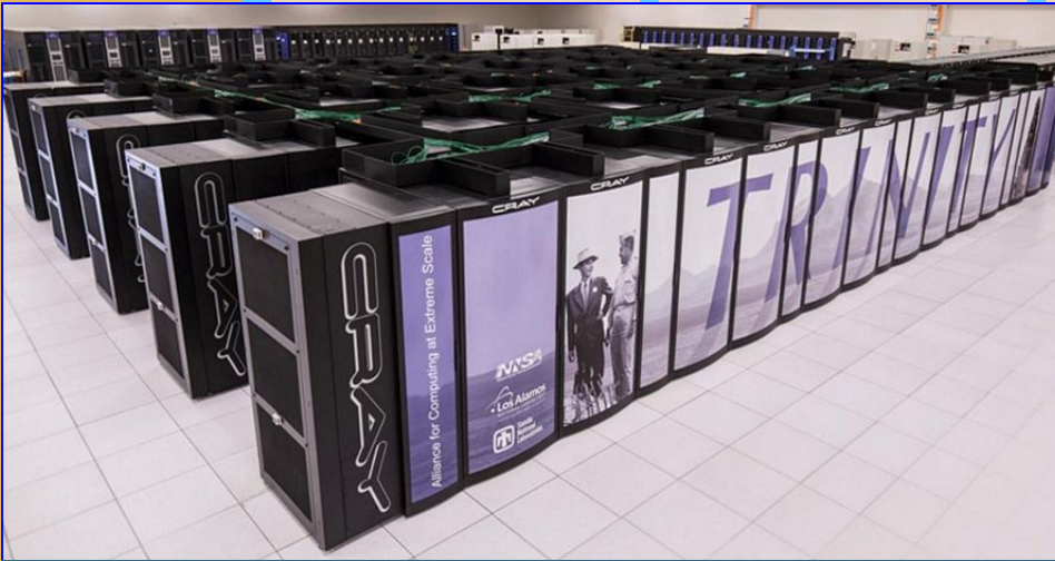
Fig. 2. The 14.14 petaflop digital computer at Los Alamos National Laboratory. A petaflop is one thousand trillion calculations per second.
