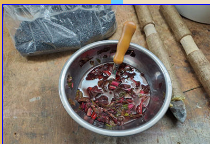
Fig. 6. This was my first experimental mixture attempt. It consisted of Hesperide vinegar with 7.5% acid + freshly harvested winter vegetables, namely chard stems + leaves with approximately 0.8% oxalic acid content.
