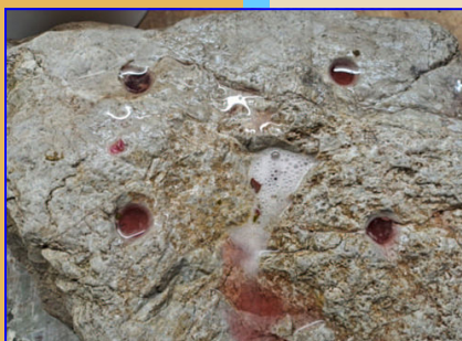
Fig. 8. In Experiment 2, I added 20% nitric acid. Detailed in the text, while some bubbling could be observed there was no sign of a jelly-like consistency to the limestone.
