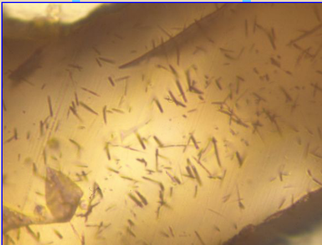
Fig.1. Photomicrograph of fission tracks in a zircon crystal from the Fish Canyon Tuff in the San Juan Mountains of southwest Colorado. The age of the zircon is about 28 million years. The longest of the tracks is about 12 microns (a micron being one-millionth of a meter) or 0.000472 inches. For reference, a single strand of hair is approximately 20 microns wide making the length of these crystals equal to about half the width of a strand of hair.
